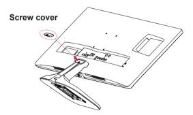
3 Remove the two screws on the back of stand body.
